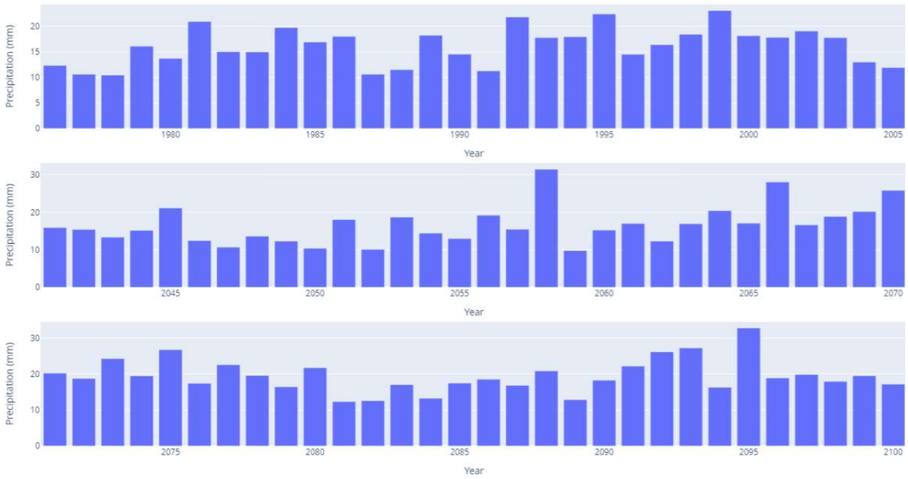
Figure 2.2: Maximum yearly 3h precipitation for RCP8.5. Top: historical period, middle: mid-century, bottom: end of century. NOTE: the years shown here do not correspond to real calendar years but rather reflect the variability and mean values of the respective periods.
