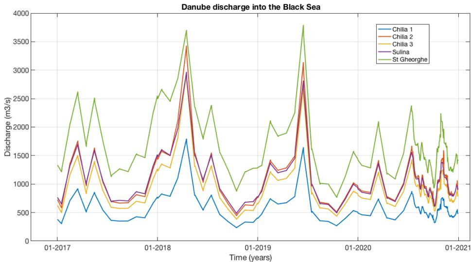
Figure 4 - Daily discharges for the Danube outlets: NIHWM interannual dataset from January 2017 until June 2020 and daily observations from July 2020 onwards as accounted in the BS-NRT model
